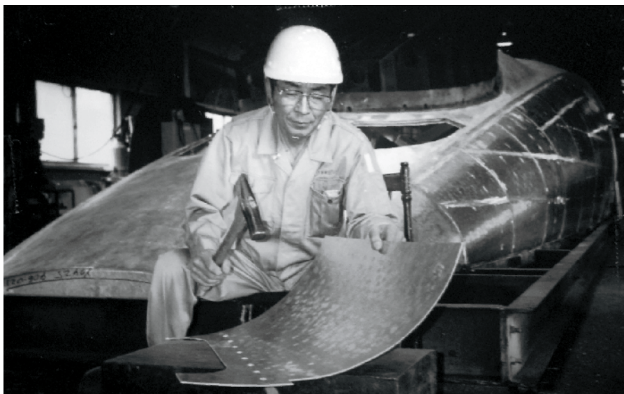
Kunimura has used the hammering technique "uchi-dashi bankin" to make the nose cones for the past 50 years at Yamashita Kogyosho. Yamashita Kogyosho collection
