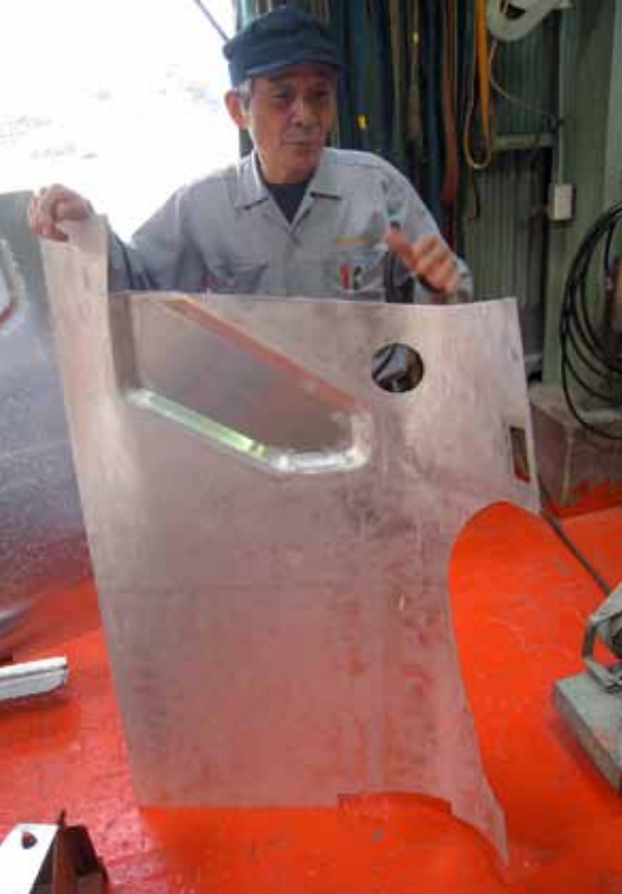
Craftsman Jiro Kunimura holds a sheet of aluminum that he hammered into shape for use in a Japanese bullet train.
