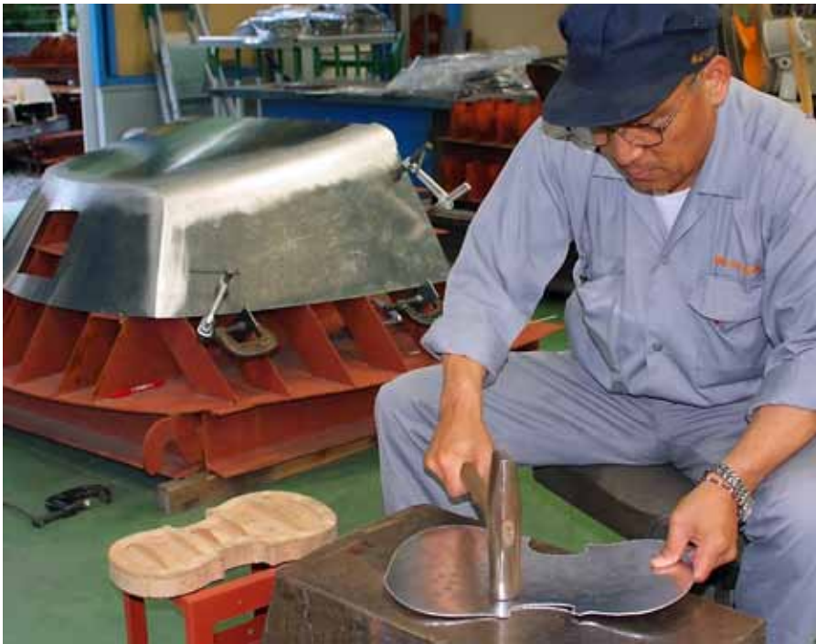
One of the company's first craftsmen, Hiroyuku Fuji crafts a hammer-made magnesium violin to show at schools to get young people interested in the craft and ultimately build the company's workforce, which is aging rapidly. Two photos, Yamashita Kogyosho collection
