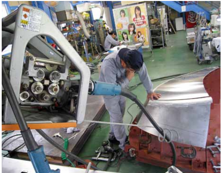
Craftsman Susumu Okada works on the cockpit of a bullet train at the Yamashita Kogyosho factory in Kudamatsu, Japan, on June 24, 2010. Workers swing their hammers in short, rhythmic strokes to soften, stretch, and mold the aluminum. Two photos, Joseph Coleman
